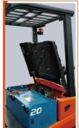
Fast replacement of the battery can meet continuous operation. The fully open hood design makes daily maintenance very convenient.
